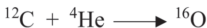
Figure 1.2. Nucleosynthesis of oxygen from reaction of a carbon nucleus and a helium nucleus
